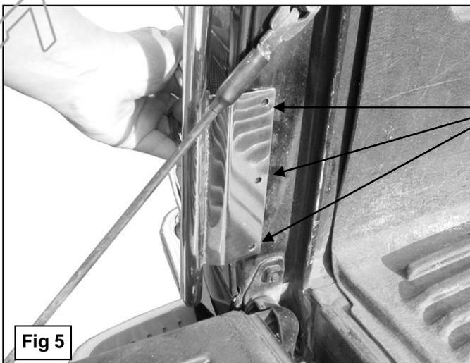
Once the three 1/8" holes have been drilled, reinstall the taillight assembly. Secure the Taillight Guard to the body panel with the supplied 5mm x 12mm Sheetmetal Screws.
